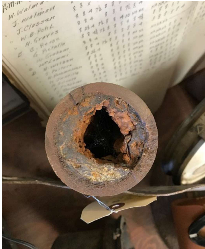
Figure 1. Photo of Tuberculation
